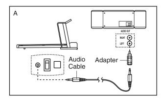
B. Plug one end of the audio cable into the jack on the front of the Incline Trainer near the power cord. Plug the other end of the cable into the LINE OUT jack on your stereo.
